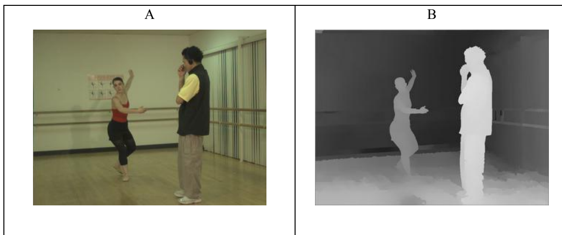
Figure 4 – (A) shows a real-life image. (B) shows a depth map regarded as “ground truth”. These images are part of the 3DTV image repository and are used in various 3DTV research projects.
