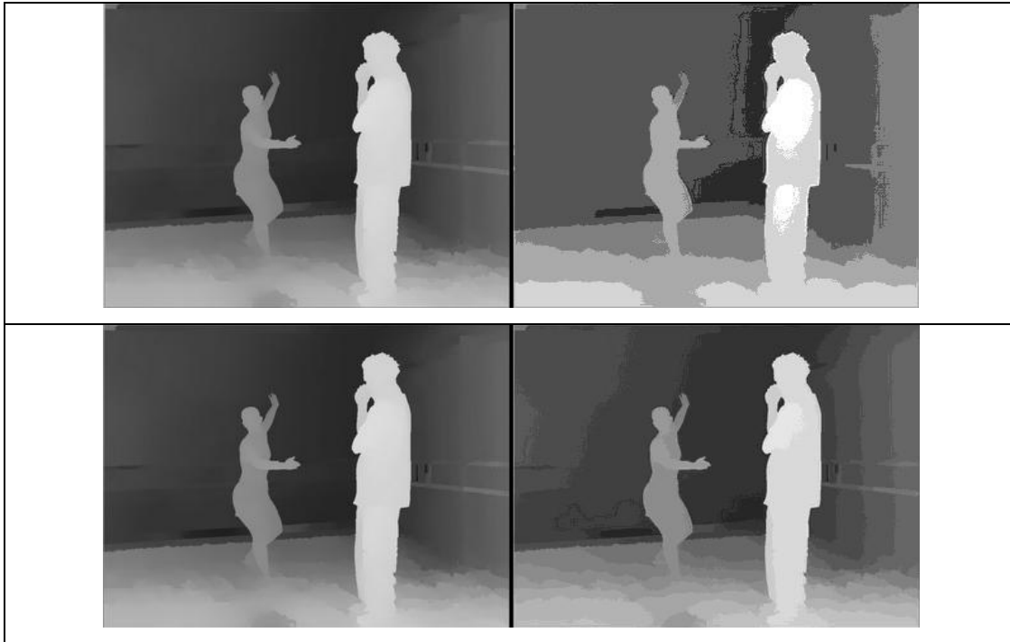
Figure 5 Top images are the “ground truth” depth map, original and quantized to 6 levels. Bottom images are the “ground truth” depth map, original and quantized to 20 levels.
