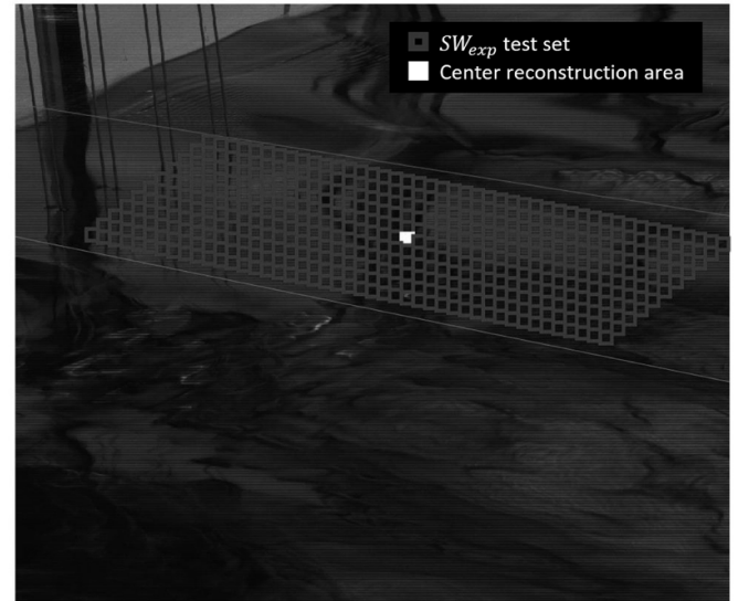
Figure 11. SW_{exp} image of AmL polarimetric reflection and the selected cells . The area between the lines is the supervised data area covered by the WG measurements.
