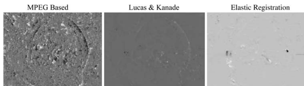
Fig. 7 Comparison of the MPEG based depth map to other commonly used optical flow method. It can be seen that the MPEG depth map contains the important motion elements that are missing in the Elastic Registration implementation. The Lucas & Kanade
