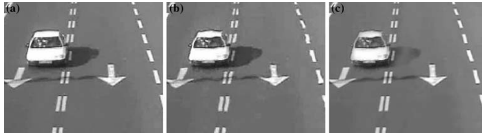
Fig. 7 Turbulence simulation and compensation. a Original sequence with real-motion and no turbulent motion; b the same frame with turbulence-like distortions induced; c the same frame after the turbulence compensation process
