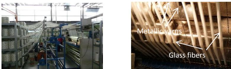
Figure1: Conductive thread insertion into warp knit.
