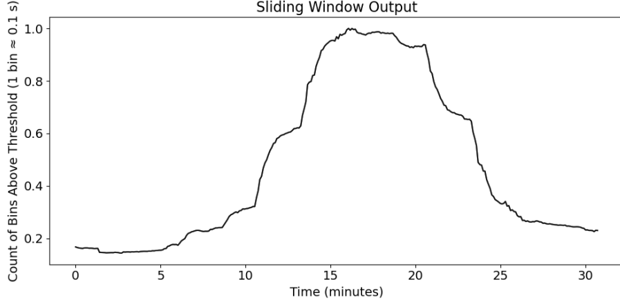
Figure 6. Sliding window aggregation of matched filter results, reflecting the temporal distribution of feeding event.
